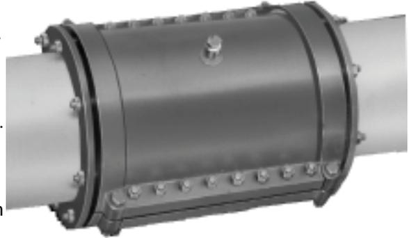
**Available in Three Styles** - the 114 MJ Split Repair Sleeve for use on straight runs of pipe and the 114 MJ Bell Repair Sleeve which is fabricated to accommodate the specific dimensions of the bell, collar or coupling to be repaired. The JCM 114 MJ Repair Sleeve can also be fabricated to accommodate two different O.D.'s of pipe.
