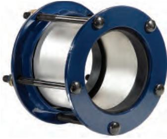
The JCM 262 Oversized Fabricated Stainless Steel Coupling provides an economical solution for joining old cast iron, larger classes of asbestos cement and other types of oversized pipe. The JCM 262 Coupling uses the popular and economical JCM G212 Transition Gasket System. Making transitions of the same nominal pipe size easy with just the change of gasket.
