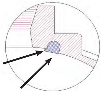
JCM incorporates this gasket design with the internal groove in the metal pipe fitting which:
