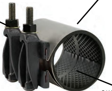
Gridded gasket with long tapered ends and recessed bridge plate assures even gasket pressure throughout range - without wrinkling or crimping. Compounded for use with water, salt solutions, mild acids and bases.
