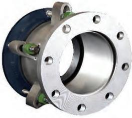
The JCM 362 Fabricated Stainless Steel Flanged Adapter provides an economical solution to join a plain end piece of pipe to a flanged fitting. Constructed of Carbon Steel End Ring with resilient Fusion Plastic Coating, a 304 Stainless Steel middle ring, flange and hardware. The JCM 362 is prepared for the harshest of elements or corrosive line content - or both!
