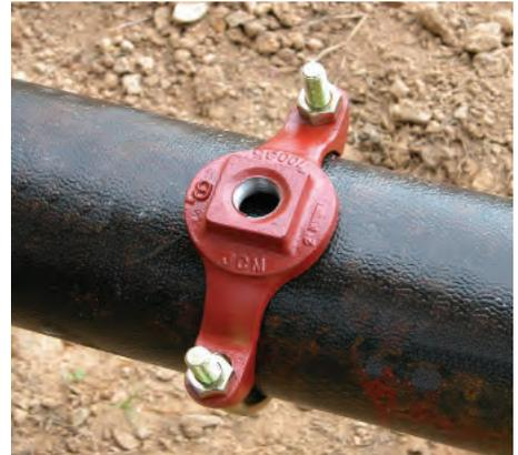
To start the JCM Service Saddle Models share a specific feature – a broad, hydromechanical-lip gasket of an acceptable durometer captured in a recessed groove around the outlet. The key working feature of a service saddle is the gasket which provides the watertight seal around the outlet area.
