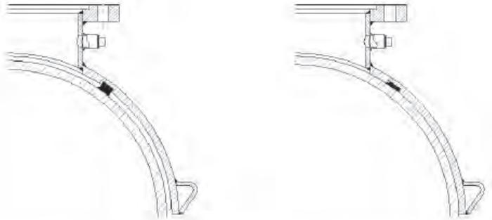
The drawing right demonstrates the system of the gasket storing and releasing energy as the pipe contracts and expands.
