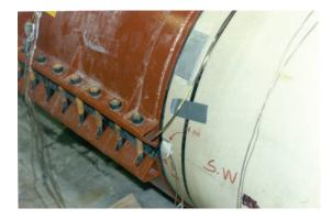
In 2013 JCM partnered with Flowtite Pipe for further evaluation of these sleeves on this pipe. A FRPM style sleeve was furnished to Flowtite Pipe engineering group. Flowtite installed, tested and evaluated a JCM 24 x 8 GRP tapping sleeve with postive results.
