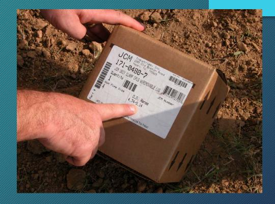
... the clamp label. If the measured O.D. of the pipe falls within the range indicated on the clamp, installation should proceed.
