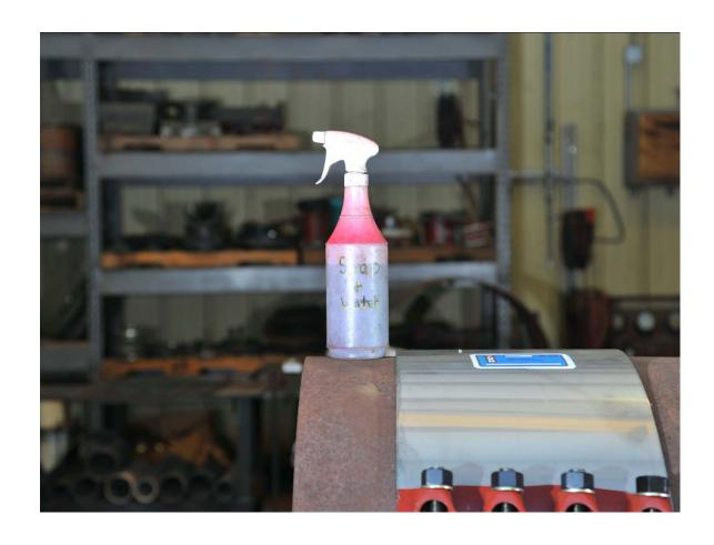
Soapy water or water alone should be used to lubricate the pipe to make installation of clamp easier. Soapy water provides a slippery surface to let the gasket slide on the pipe into place and is water-soluble. Do Not Use Oil Base Pipe Lubricant – it does not break down with water and will not allow the gasket to adhere to the pipe for water tight seal.
