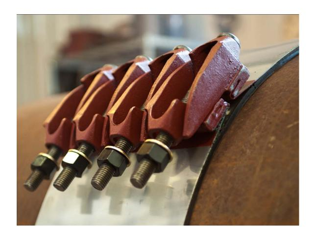
To ease installation, loosen the nuts (do not remove) on the other lug bolt units and open the gap between the two halves. When clamp is installed, all lug units should have approximately the same space between lug halves.
