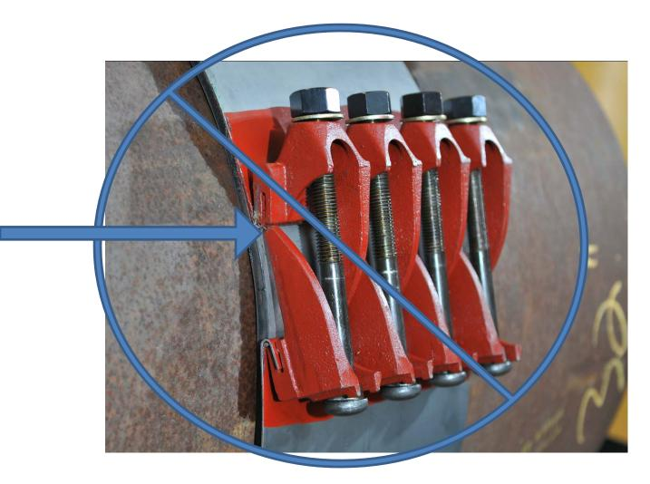
Be aware of the ends of the finger lug and ensure that they overlap the opposing lug and not interfere with the lug bar.
