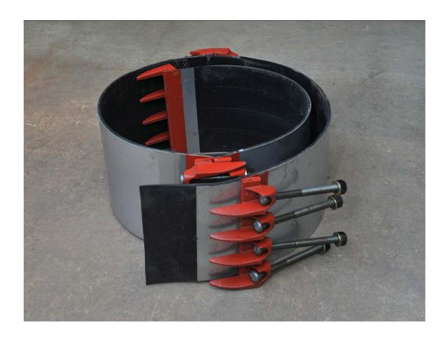
JCM 102 Multi Band Clamps 10" (254mm) and larger are manufactured with heavy duty stainless steel (minimum 17 gauge) and substantially larger lug units and 3/4" (19.05mm) bolts & nuts. These clamps are robust in weight and materials and will withstand rugged installation.
