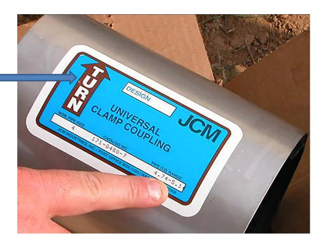
JCM Universal Clamp Couplings include a feathered, tapered gasket edge that lies flat beneath the clamp that completes the full circle gasket. It is critical that these tapered gaskets lay smooth under the stainless steel band. Multi Band Clamps have a feathered gasket on each section. To assist the tapered edges to be smooth, the clamp should be rotated in the direction of the arrow on the labeling on the clamp.
