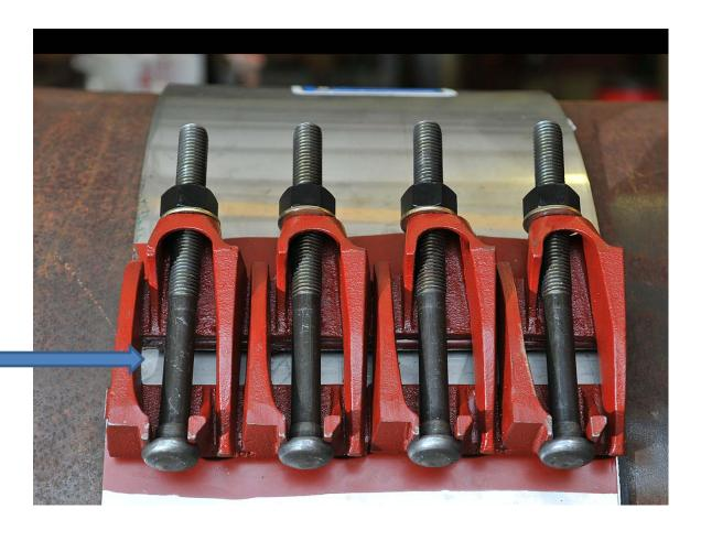
When tightening is completed, each clamping lug section should have an approximately equal gap between lug sections. **Tighten All Bolts Evenly to the following values:**
