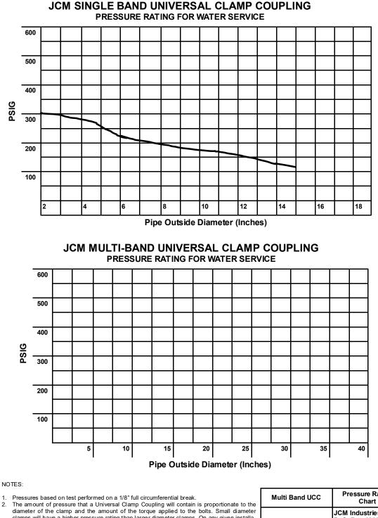
diameter of the clamp and the amount of the torque applied to the bolts. Small diameter clamps will have a higher pressure rating than larger diameter clamps. On any given installation, the pressure capability of a clamp is heavily influenced by the type and extent of the damage, service conditions, site conditions and installation workmanship.
