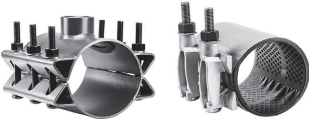
Figures 1A and 1B. As pipeline size and pressure increase, a tapping sleeve or repair sleeve with a thicker body and a contained outlet gasket seal (left) can provide better mechanical alternatives for increased pipe support, added hoop strength for the pipe, and increased pressure-holding capability than a fitting with a full circumferential gasket and a thinner, more flexible body (right).
