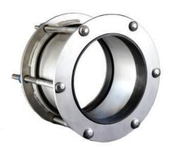
Purchase orders for the JCM Industries, Inc 6262 type coupling signify an agreement between the manufacturer and customer that both parties agree to the JCM test procedure for meeting ANSI/AWWA C219 Standard for Bolted, Sleeve-Type Couplings for Plain-End Pipe. All couplings are pneumatically tested to a minimum of 25 PSI. Additional testing for certification purposes available upon request with additional charge.
