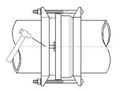
4) Slide the casing gland onto the inner serrated ring. Insert oval-neck bolts through corresponding gland holes and tighten to 65 ft./lbs. Hammer-set the casing gland (that is positioned over the inner serrated ring) at several places around the gland and tighten the nuts to 150 ft/lbs.
