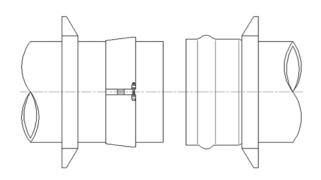
In order, slide the second casing gland and inner serrated ring onto the pipe spigot - connect the bell and spigot per standard pipe installation practices.
