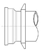
1) Slide one casing gland down the pipe barrel to seat against the bell slope (larger opening toward bell).
