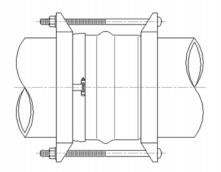
4) Slide the casing gland onto the inner serrated ring. Insert oval-neck bolts through corresponding gland holes and tighten to 65 ft./lbs.
