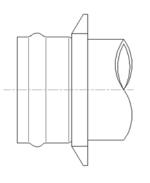
1) Slide one casing gland down the pipe barrel to seat against the bell slope (larger opening toward bell).
