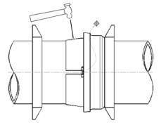
3) Position inner serrated ring against the bell face and remove the wooden spacer; tighten the positioning pin firmly (using allen wrench provided) until ring seats securely on pipe. Hammer-set inner serrated ring at several places around ring and re-tighten the positioning pin firmly.
