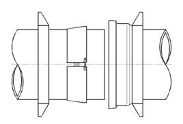
In order, slide the second casing gland and inner serrated ring onto the pipe spigot - connect the bell and spigot per standard pipe installation practices.
