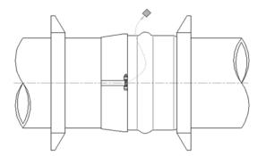
Position inner serrated ring against the bell face and remove the wooden spacer; tighten the positioning pin firmly (using allen wrench provided) until ring seats securely on pipe.
