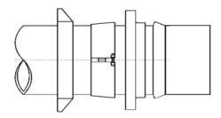
Install, in order, onto pipe spigot: casing gland, inner serrated ring, mechanical joint follower gland and gasket.
