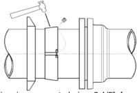
3) Position inner serrated ring 2-1/2" from MJ gland, adjust serrated ring restrainer square with pipe and remove wooden spacer, tighten positioning pin firmly (using allen wrench provided) until ring is secure on pipe. Hammer-set inner serrated ring at several places round the ring and re-tighten the positioning pin firmly.
