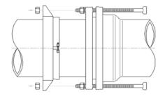
4) Insert the extra long T-Bolts through the MJ fitting and gland. After placing a nut behind the follower gland, align the bolts through the casing gland. Tighten the back (second) nut to 65 ft./lbs.
