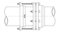
5) Install the remaining MJ bolts and evenly tighten all follower gland nuts to AWWA standards for mechanical joints.
