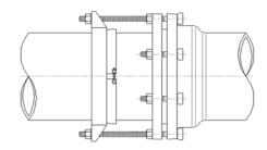
5) Install the remaining MJ bolts and evenly tighten all follower gland nuts to AWWA standards for mechanical joints.
