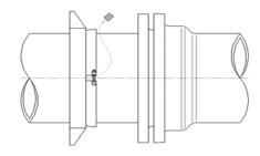
3) Position inner serrated ring 2-1/2" from MJ gland, adjust serrated ring restrainer square with pipe and remove wooden spacer, tighten positioning pin firmly (using allen wrench provided) until ring is secure on pipe. Slide casing gland forward to seat onto the inner ring.
