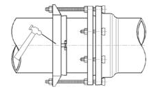
5) Hammer-set the casing gland at several places around the gland and tighten the back nuts to 150 ft/lbs.
