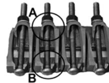
Open clamp at open ear lug segment and place clamp on pipe. Bring back half of clamp around pipe. Mesh top lug fingers into "open ears" and engage bolts. Finger tighten bolts to hold in place. Begin tightening bolts to proper torque values. Continue around pipe at each lug segment. Avoid tightening lugs to metal bound at any one segment - *gaps between lugs should be approximately even on both sides. Continue bolting sequence to proper torque values below.*
