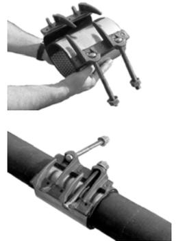
**Multi Band Clamps** - with multi lug segments. One section has "closed ears" (A) and "open ears" (B) for bolt engagement. Locate lug segment with open "ear" to loosen bolts. Loosen bolts of other lug segments. Do not remove bolts.
